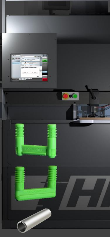
The HPLD is a horizontal point to point Lockdowel inserting machine. This machine will insert H-clips, Channel Locks and Spring Pins with ease.
