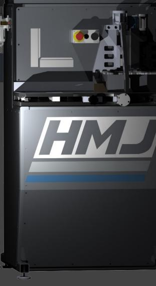
The HMJ is a CNC machining center used for producing high quality Haunch Joints which are used in many furniture and cabinetry applications. The haunch head miters the profile for beaded face frame applications on both stiles and rails.
