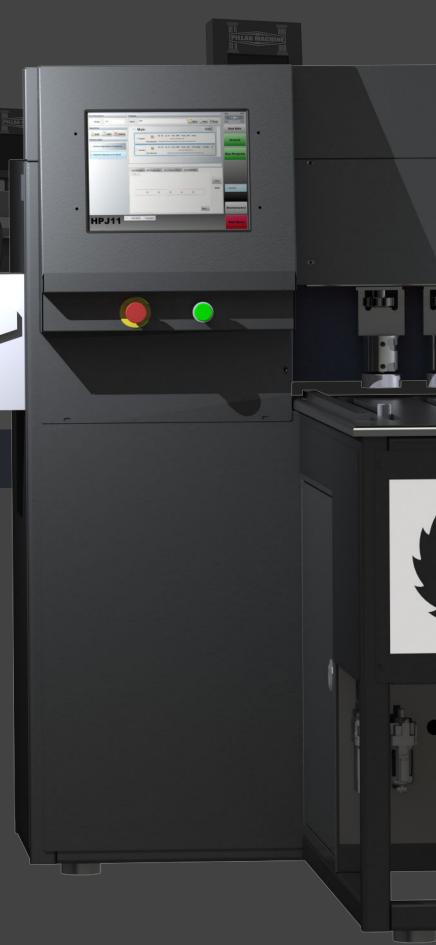
The 2S is a multi-axis, mulit-functional CNC horizontal machine. It is designed to size and square edge glued panels safely and accurately. The 2S can also be Pillar-Linked to any order entry program to scan barcodes. This will virtually eliminate the need for the operator to do anything other than load the part to be cut.
