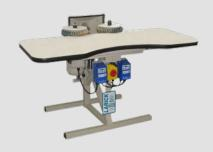
The Model 220 Profile Sander is a two spindle machine designed for use with flexible brush type sanding wheels. The spindles are counter-rotating, allowing corners to be sanded without rounding over, and to sand in two directions. There are two height settings, allowing it to be used for both edge and panel sanding. In the raised position, the table moves toward the spindles, under the panel sanding wheel, providing support for small panels.
