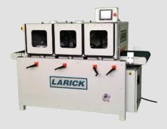
The LARICK 6000 Series machine will brush sand and/or wire brush parts with standard widths from 25 to 73 inches. It has 1 to 6 spindles which will accommodate sanding or wire brushes up to 14 inch diameter. It has a fixed height conveyor and accommodates parts up to 9 inches thick.
