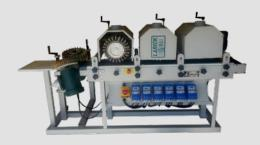
The 700 series sander has a variable speed conveyor under the top sanders. It can be configured with 2, 3, or 4 top sanding spindles, and with or without universal side sanding stations. The conveyor can be either 9 or 15 inches wide.
