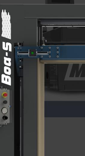
The Boa-S is a manually operated Case Clamp designed to clamp cabinet boxes, drawer boxes and case goods that have been doweled together. This version of the case clamp is servo assisted in both horizontal and vertical clamping, making it simple to manually move into position. Since the Boa-S is manual, you can quickly and easily transition between box sizes without needing to wait for slow moving clamp parts.
